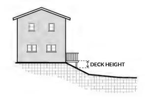
FIGURE 18.02.030.C.2: MEASURING HEIGHT OF DECKS
