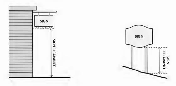
FIGURE 18.18.050.C: MEASURING SIGN CLEARANCE
