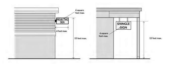
FIGURE 18.18.090.C: PROJECTING AND SHINGLE SIGNS
