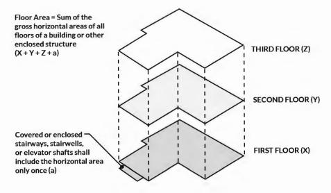
FIGURE 18.02.030.E: DETERMINING FLOOR AREA
