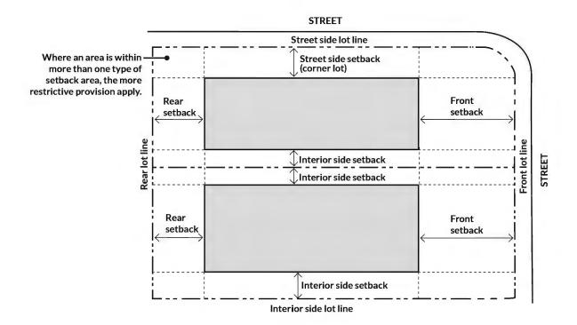
FIGURE 18.02.030.I: DETERMINING SETBACKS
