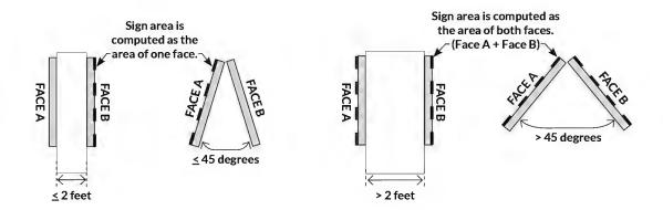
FIGURE 18.18.050.A.2: MEASURING SIGN AREA, DOUBLE-FACED SIGNS
