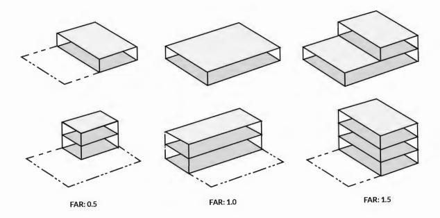
FIGURE 18.02.030.F: DETERMINING FLOOR AREA RATIO
