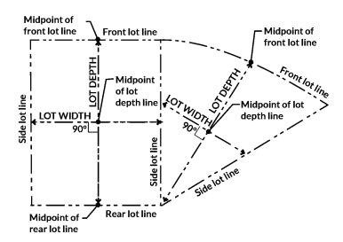
FIGURE 18.02.030.D: MEASURING LOT WIDTH AND DEPTH
