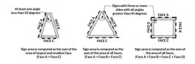
FIGURE 18.18.050.A.3: MEASURING SIGN AREA, MULTI-FACED SIGNS
