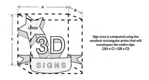
FIGURE 18.18.050.A.4: MEASURING SIGN AREA, 3D SIGNS
